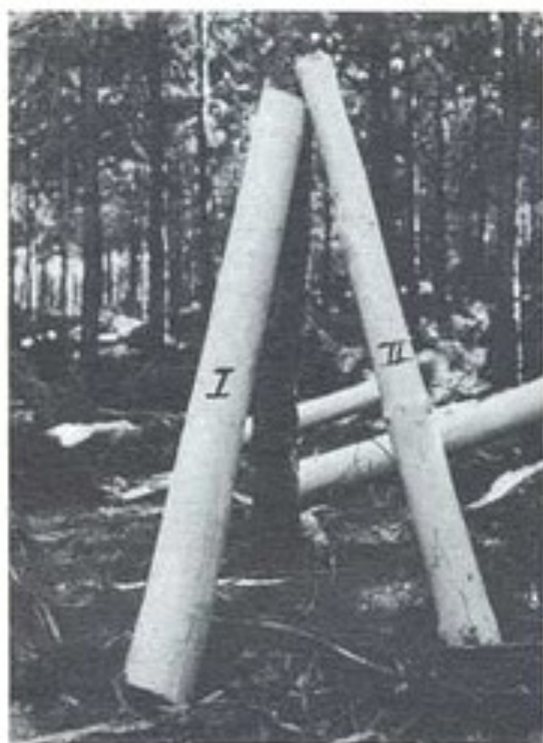
Red pine posts cut in thinning 1950. Planted 1927. Post I pruned 1945. Post II unpruned
